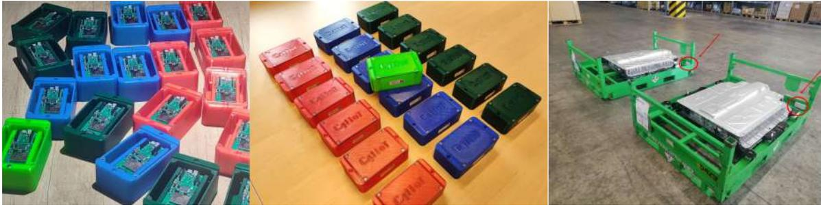
The devices perform measurements by reading the on-board sensors (GPS data, acceleration and magnetic field from the IMU chip, and the temperature), as well as the anomaly detection inference results as calculated on the edge nodes. The data is transmitted to the Field Gateway using NB-IoT connectivity, or GPRS in cases when there is no NB-IoT network available. The format of the binary data which is transmitted in UDP packets is as follows:
